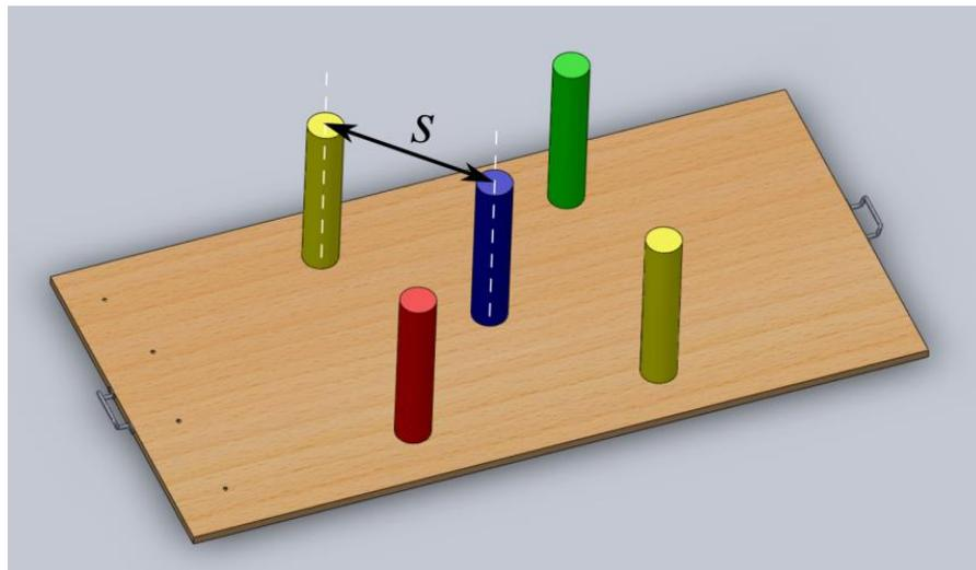
FIGURE 4: CONGESTED ENVIRONMENT TILE. THE RUBBER TUBES ARE MOVED TO MATCH ROBOT DIMENSION.
